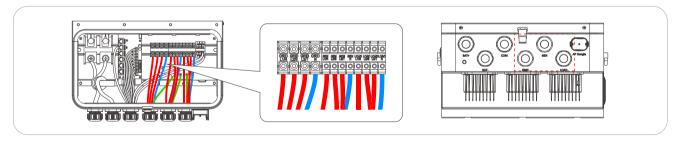
NOTE: Please ensure that the N and L wires are connected accurately.
