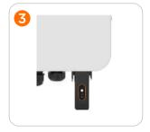
NOTE: When the AP Dongle is powered on normally, the green light remains on. When connected to WIFI, both the green and blue lights will remain on.
