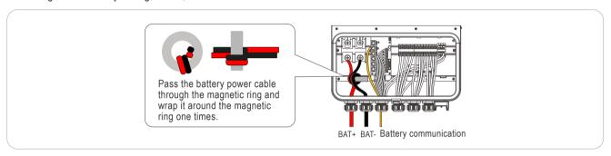
NOTE: Ensure that the polarity of the battery and PCS are correctly connected, otherwise PCS may be damaged.
