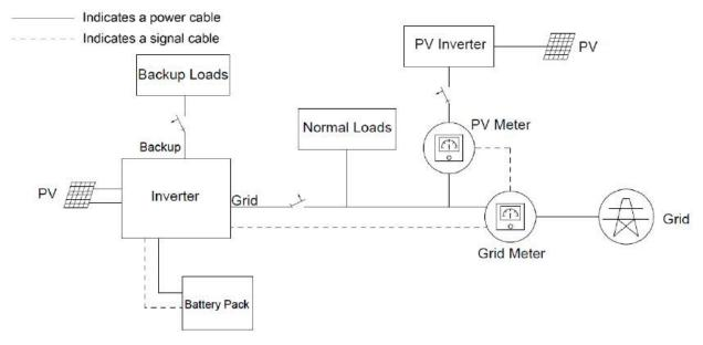
Brief wiring diagram of the hybrid-coupled system
