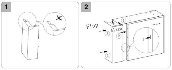
Disassemble the cable cover of the battery SMILE-G3-BAT-3.6S/4.0S
