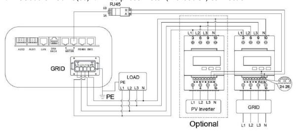
Meter communication cable requirements: two-core outdoor shielded twisted pair copper cable (flexible), conductor cross-section 0.5~1.5mm², wires terminal should be fitted with bootlace ferrules.
