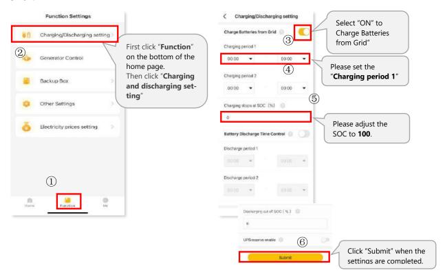
If the formula "Grid Power≈ **Load** + Battery Charging Power" fits well, the grid meter installation of the energy storage inverter is correct. Please remember to deactivate the "Charge Batteries from Grid" by clicking "OFF" and save the changes.
