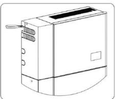
c. Align the hooks on the right side of the cable cover to the slots on the front cover side, downwards insert the cable cover along the edge of the inverter front cover.
