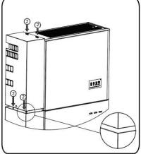
Disassemble the cable cover of the energy storage inverter
