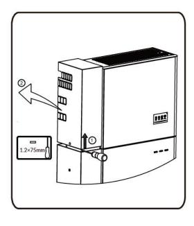
Mount left cable cover and right cover of the inverter when inverter mounting with wall bracket, please follow the steps below.
