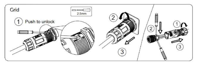
Disassemble the backup plug connector (e.g. due to faulty assembly), proceed as follows.
