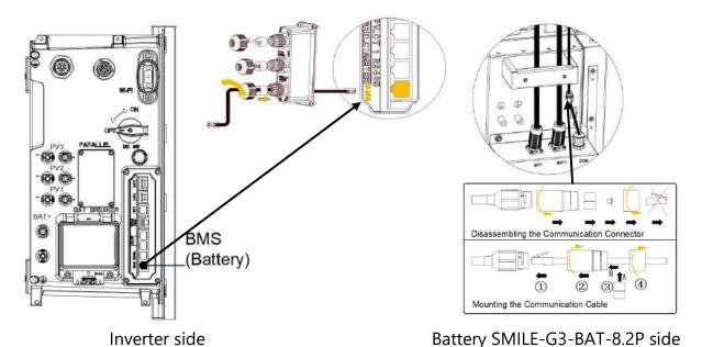
Communication cable connection between the energy storage inverter and series batteries:
