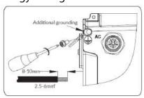
Grounding connection between the energy storage inverter and series battery.
