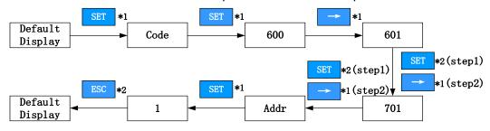
When the meter is used as PV meter, please follow the steps below to complete the address setting:
