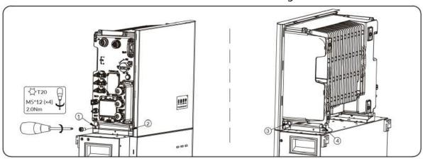
Mount the inverter with wall bracket for battery ready scenario.
