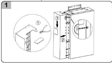
Disassemble the cable cover of the battery SMILE-G3-BAT-8.2P
