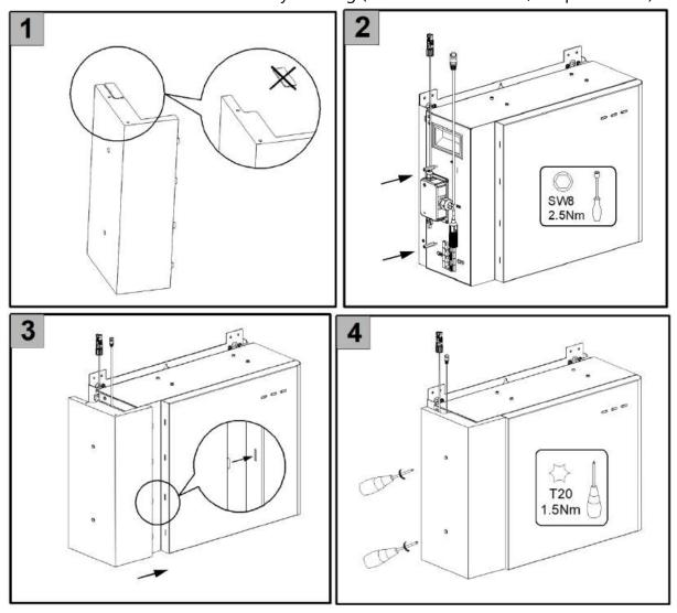
Disassemble the cable cover of the battery SMILE-G3-BAT-3.8S
