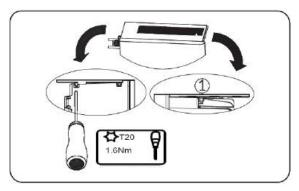
Mount left cable cover and right cover of the inverter when inverter standing on the battery, please follow the steps below.
