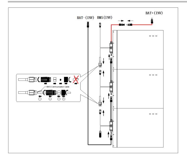
Cables connection between the Inverter and series batteries of two column.
